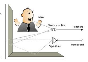
video call can be speaking and interacting simultaneously. This ability to continuously transmit sound in two directions is called full-duplex audio. Many speakerphones on the market cancel echo simply by muting one person's microphone while the other is speaking. This often results in frustrating, broken, and unnatural conversations - similar to the experience of talking on a walkie-talkie.
